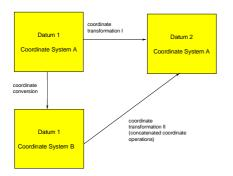
Annex 2 contains the schema with the elements describing a coordinate operation in the case of coordinate transformation (example: transformation from German geodetic datum DHDN to ETRS89).
